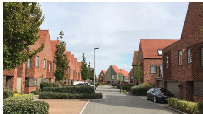
Figure 52: Street designed with parking located in front of homes and screened with robust shrub planting and small trees. Planting is kept low to maintain visibility along the street and towards front doors. Horsted Park, Kent. Source: National Design Guide.
