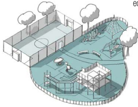
Figure 73: Types of play space: local areas of play (LAP), local equipped areas of play (LEAP) and neighbourhood equipped area of play (NEAP). Source: National Design Guide, part 1.
